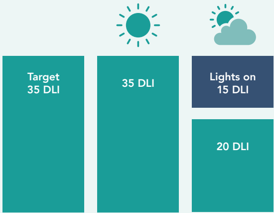
The Argus DLI program supplements the exact amount of artificial light required
