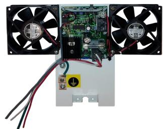
The ACM is used for distributing the heat load within electrical panels whenever the electrical components are dissipating considerable amounts of heat and when the panels are installed in warm locations.
