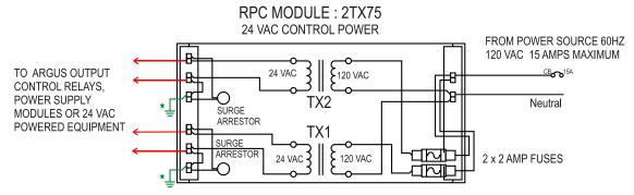
\* Transformer secondary to be grounded unless powering a Titan IO Power Supply or other equipment in need of isolation.
