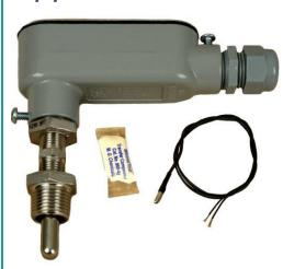
The SEN-TN2DW/C assembly can be used for pipe and tank temperature measurement in heating, nutrient control, and irrigation applications. The custom dry well enables sensor replacement without the need for draining the system. A standard Argus TN2 sensor is included.
