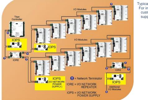
Typical Wiring Configuration For installation, refer to the custom wiring diagrams supplied with each part.
