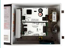
The I/O Network Repeater is used to regenerate the digital communications signal on I/O network wire runs more than 300 meters and whenever a branch in the network wiring is required.
