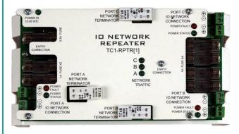
The I/O Network Repeater is used to regenerate the digital communications signal on I/O Network wire runs more than 300 meters and whenever a branch in the network wiring is required.
