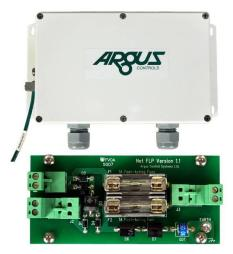
A separate NFLP module is installed at each end of exposed Argus Titan network sections. In the event of excessive lightning energy coupling into the exposed network section, the fuses on the NFLP are designed to blow, isolating the rest of the network from the surge and safely discharging the lightning energy to ground.
