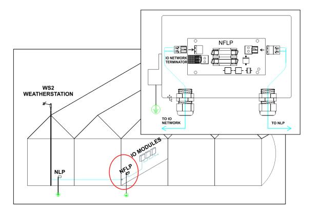
Typical wiring example. For installation, refer to the supplied wiring diagrams and instructions.
