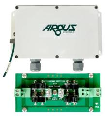
The NLP (Network Lightning Protection) module provides additional protection from substantial lightning surges while allowing power & communication signals to pass under normal conditions. It is typically installed on the I/O communications network between the highly exposed weather station (TC-WS2) and the NFLP (Network Fused Lightning Protection) module used to protect the rest of the I/O hardware on the network (refer to the Argus Data Sheet TC-NFLP-1.0/C for additional details).
