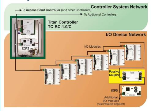
**Typical** placement of a Passive Coupler on an I/O Communications Network
