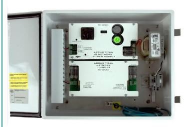
Passive Couplers are conveniently configured to power one I/O network segment and provide power and lightning transient isolation in one easy to install package. Only the I/O network communications signal passes through the Passive Coupler device unchanged.
