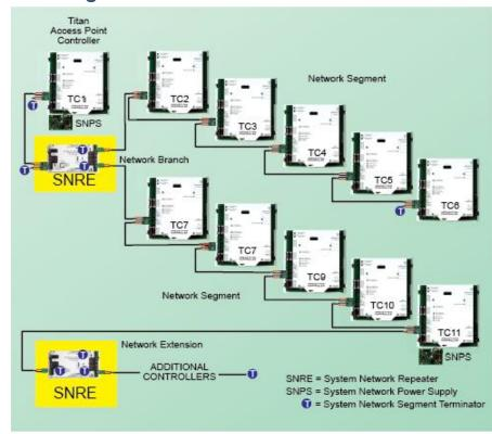
Typical placement of System Network Repeaters on a Multi-Controller Titan System.
