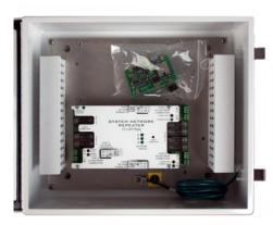
The System Network Repeater is used to regenerate the digital communications signal on system network wire runs more than 300 meters and whenever a branch in the network wiring is required.
