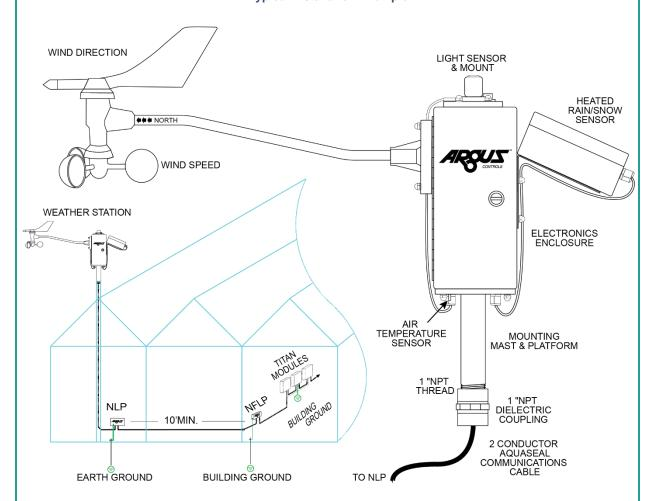
Typical wiring example. For installation, refer to the supplied wiring diagrams and instructions.
