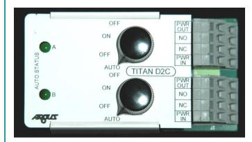
The **TTN-D2C-1.0/C** Output Relay board can control up to 2 digital devices.
