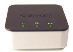
The Obi adapter is an **add-on device** connecting to your analog automatic dialer to give it VoIP access. It cannot work on its own.
